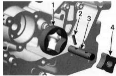
1. Outer rotor 2. Needle pin 3. Oil pump shaft 4. Inner rotor
