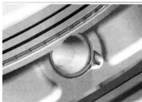
CORRECT POSITION OF THE PISTON CIRCLIP
